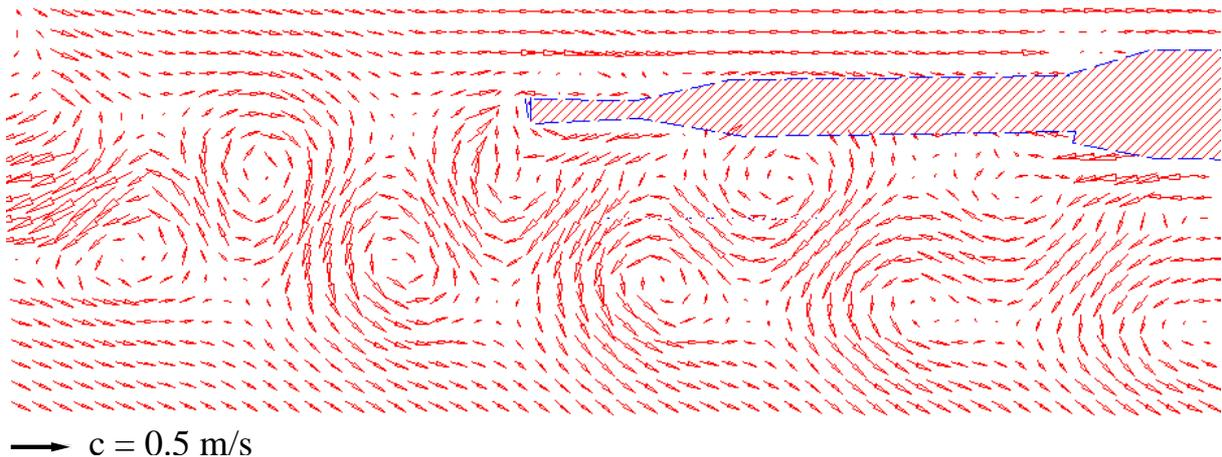
Abb. 1: The field of the velocity vectors as PIV results <sup>1</sup>
